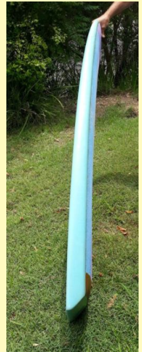
(b) Frank Latta bellyboard: 1700 x 500 x 75 mm. Nose 420 and tail 370 mm.
