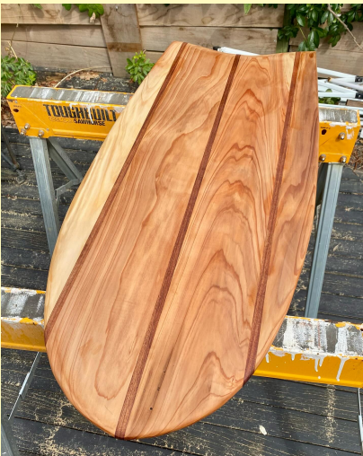
(a) Japanese Cedar with Tasmania Black wood, finish with homemade beeswax polish.
