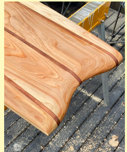
(b) 12mm central concave, with 80mm wide 10mm deep chines to the rails.
